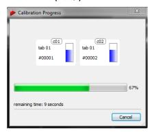
After a successful room calibration, the DTrack2 info window with the calibration results is displayed. The number of valid frames should be greater than 70% for each camera.
