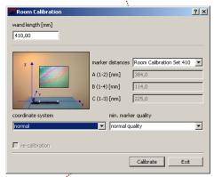
Press "Calibrate" and the calibration starts within 5 seconds.
