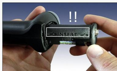
Apply the cover of the battery compartment and fix the screw again.
